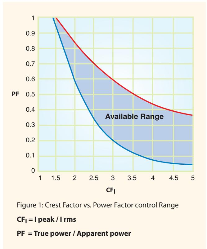
As seen in Figure 1, for a crest factor of 1.414, the programmed power factor can only be 1 if the input voltage is a sine-wave. However, for a CF of 2.0, the acceptable PF ranges from 0.608 to 0.85; for CF = 3, the PF can then be set from 0.211 to 0.6, etc. So, higher crest factors enable a wider range of power factors.
