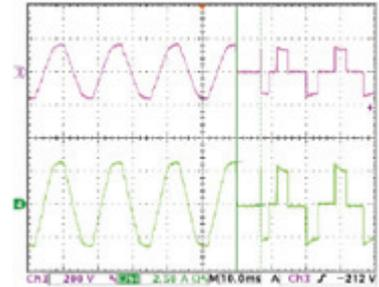
Figure 7 : Transfer time for Off-Line UPS
